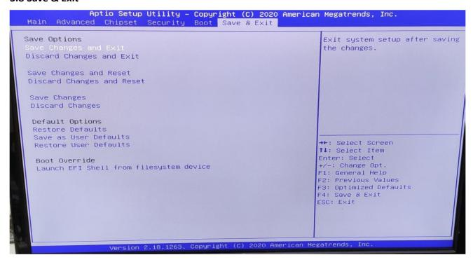
This screen provides functions for handling changes made to the BIOS settings and the exiting of the Setup program.
