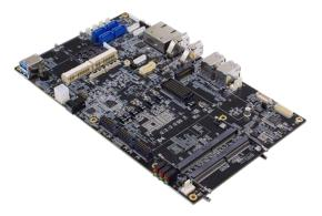
The 3.5 EBX SBC OXY5741A provides extraordinary computing performance under extreme environment. It is powered by 9th/8th Gen Intel® Xeon® / Core™. Featuring Intel's Xeon E-2276ML and ruggedized open-standard EBX architecture, 7Starlake EBX series is built tentatively and triumphs on environmental testing. It still operates effectively under harsh environments ranging from -40 to 85°C so that it is a perfect
