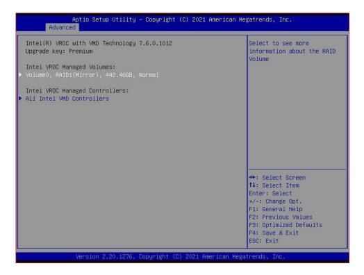
Install the VMware ESXi on to VMRAID as shown in the following example:
