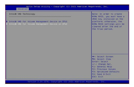
Enable the "VMD" for RSC-R1UW-2E16 that contains the M.2 NVMe devices. The other two VMDs will remain disabled.
