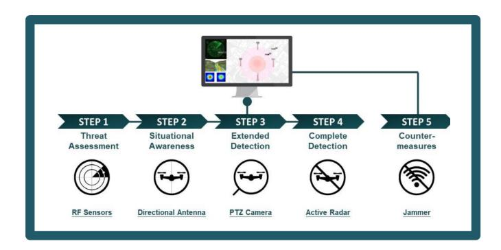
This system outlines the architecture and operational flow of a modern C-UAV system, highlighting a four-step process: **Threat Assessment**, **Situational Awareness**, **Extended Detection**, and **Counter-Measures**. Each step integrates advanced technologies and sensor fusion to ensure a robust and responsive defense against unauthorized drone activity.
