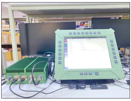
The USB interface is used to transmit the side-panel function-key signals of the display.
